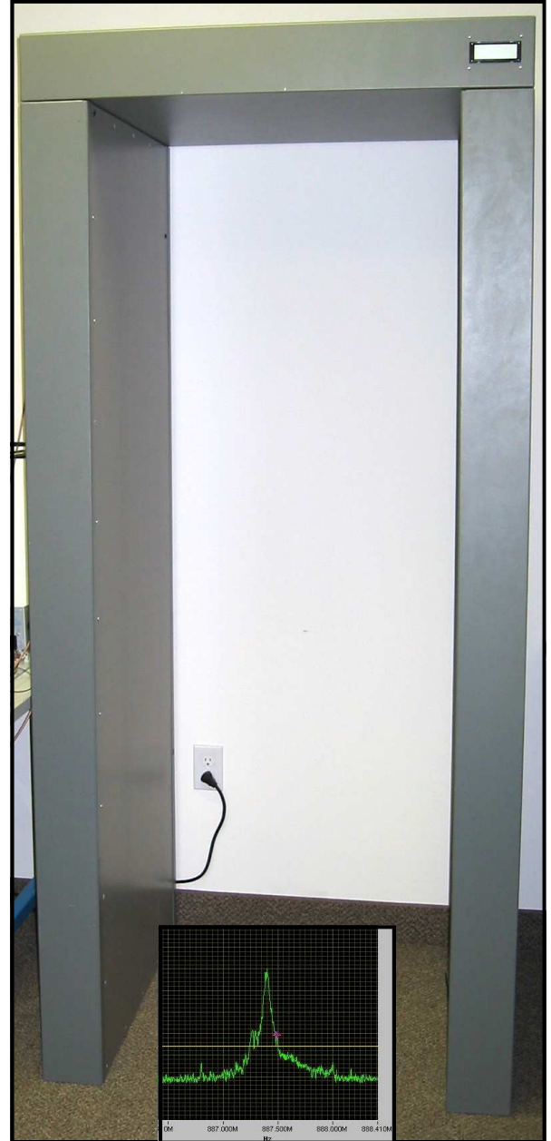
Actual detection of a cellular phone, with the battery removed, displayed on a spectrum analyzer
